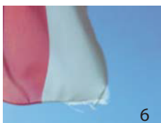
6 The first significant damage appears on the outer edge (seam and material).
